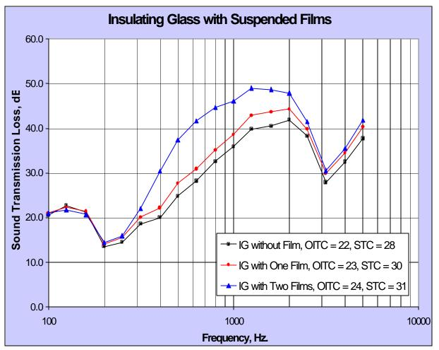
Figure 3.5 - Suspended films in insulating glass units
