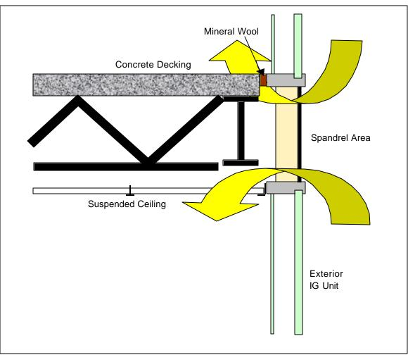
Figure 1.7.3 - Flanking Paths for a Curtain Wall Assembly
