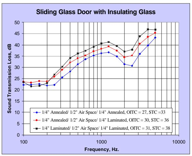
Figure 3.2 - Annealed versus laminated glass performance
