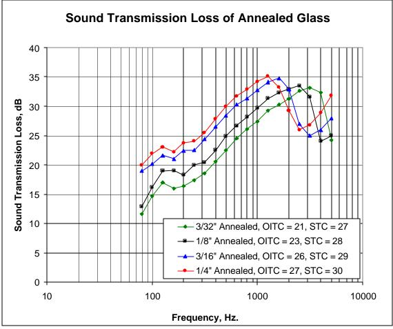
Figure 1.6.1 - Coincidence Dip for Various Glass Thickness
