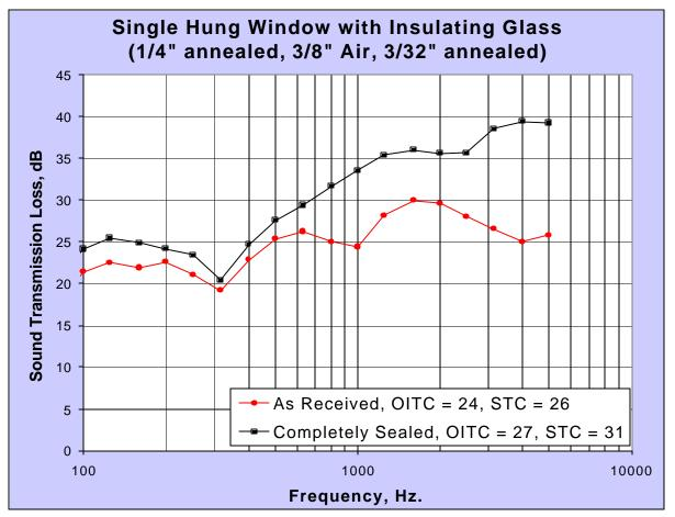
Figure 4.1 - Air Leakage Effect on Sound Transmission Loss
