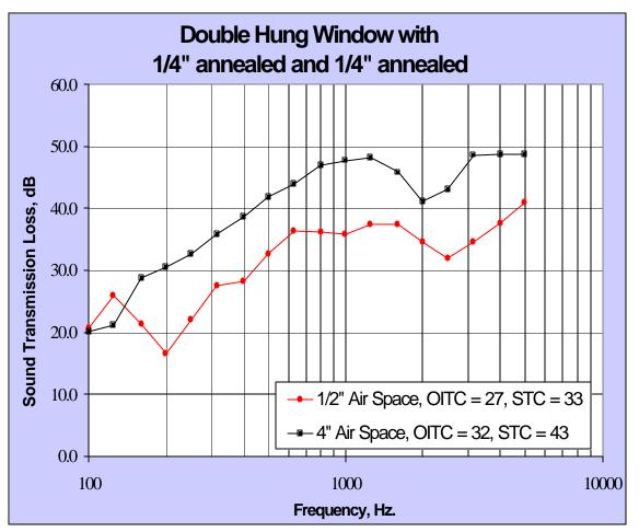
Figure 3.4 - Air Space Effect on Sound Transmission Loss
