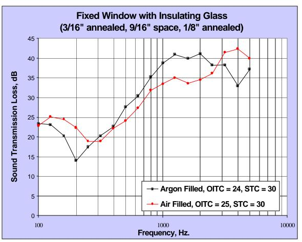
Figure 3.6 - Gas fill effect sound transmission loss
