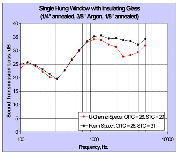
Figure 3.7 - Spacer Effect on Sound Transmission Loss
