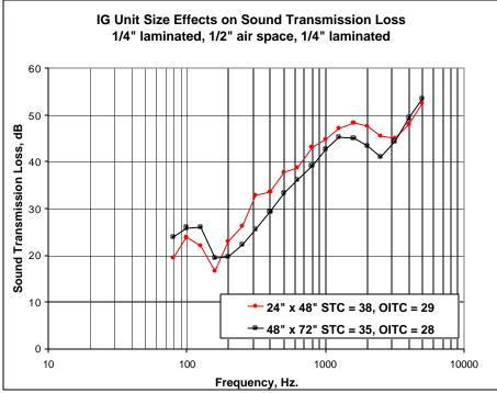
Figure 3.9.1 - Glass Size Effect for Annealed Glass
