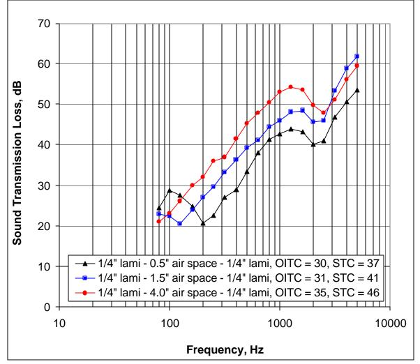
Figure 1.6.2 - Shift in Mass-Air-Mass Resonance with Larger Air Spaces
