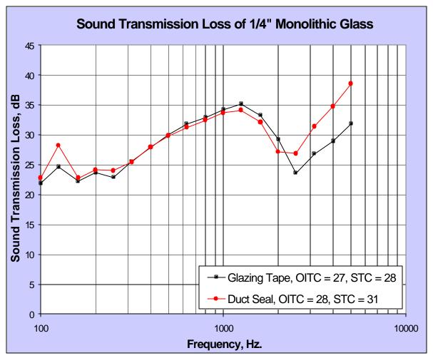
**Figure 3.8 - Edge Damping Effect on Glass Panels**
