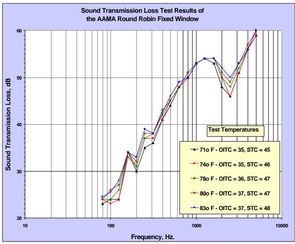
**Figure 3.3 - Temperature effect on laminated glass**
