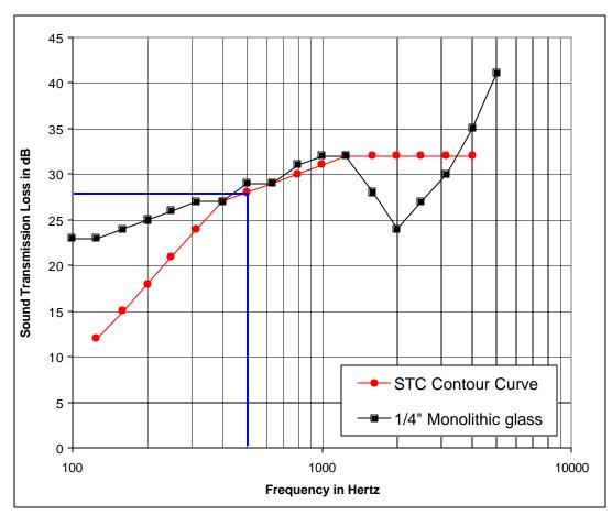
Figure A1.1 - Typical STC Contour (STC-28).
